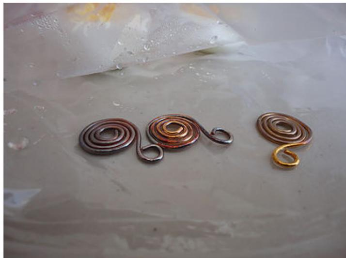
The gas tests were only slightly less effective in the first hour. In fact, with the boiled egg in a Ziploc, you can she got quite a bit of change just in the first 30 min. For those of you wanting to try to patina metals, this is a perfect method to achieve a rainbow of colors on all three metals very inexpensively. Liver of Sulfur will produce the same effects, but in a much shorter period of time.
