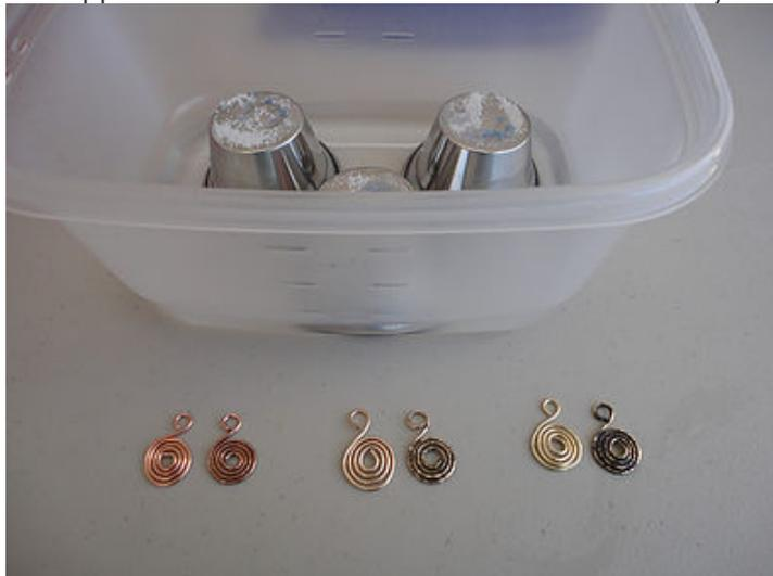
Results also showed up pretty quickly with ammonia gas . The last two tests in outdoor air and bleach gas had no change at the end of one hour.
