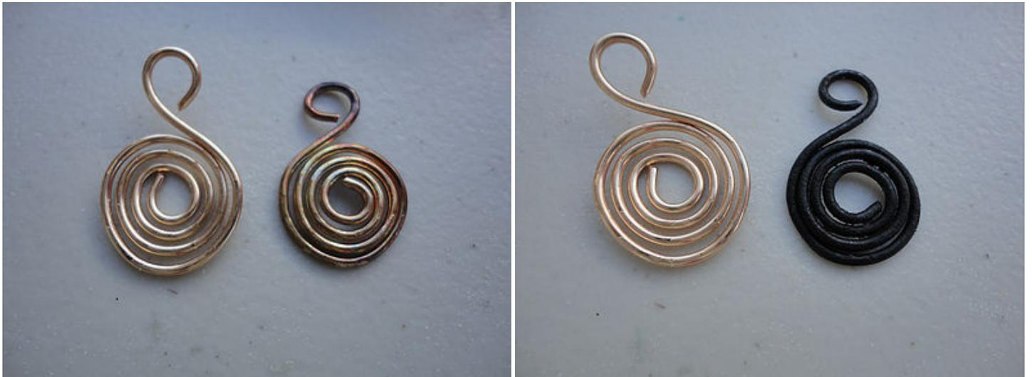
Bronze antiques quite well with a boiled egg, but turns solid deep black in Liver of Sulfur (similar to the picture below). Bronze turns black in ammonia gas. I'm curious to do this experiment over again and toss it in to the tumbler to see how much black I can keep while adding a shine! In liquid ammonia, bronze barely changed at all. It only appears to be slightly darker, but not enough so to use in jewelry preparation.
