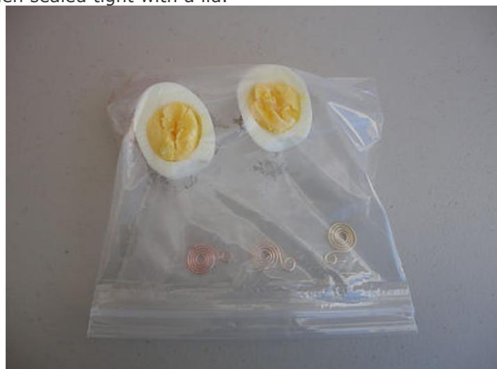
The sulfur gas was produced from a boiled egg inside of a ziploc bag.
