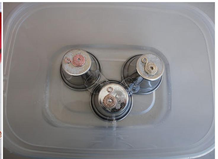
Next, each of the "pendants" were placed into their testing containers and labeled. The liquid tests were done inside disposable plastic cups. For most of the items being placed in a gas, we poured each chemical in a medium sized Tupperware and turned three small stainless containers upside down inside the fluid to create platforms for each piece of metal. These platforms allowed the pendants to stay and out of the chemical liquid. The entire container was then sealed tight with a lid.
