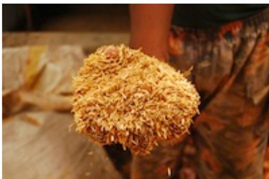
Rice Husk: Rice husk is procured from mill. It is mixed with soil as clay tends to break while drying. It also prevents the cracking of mould during firing.
