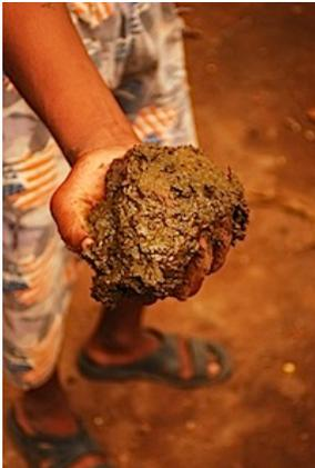
Cow-Dung (Gobar): It is mixed with river soil, which allows the wax to melt out of the cast.
