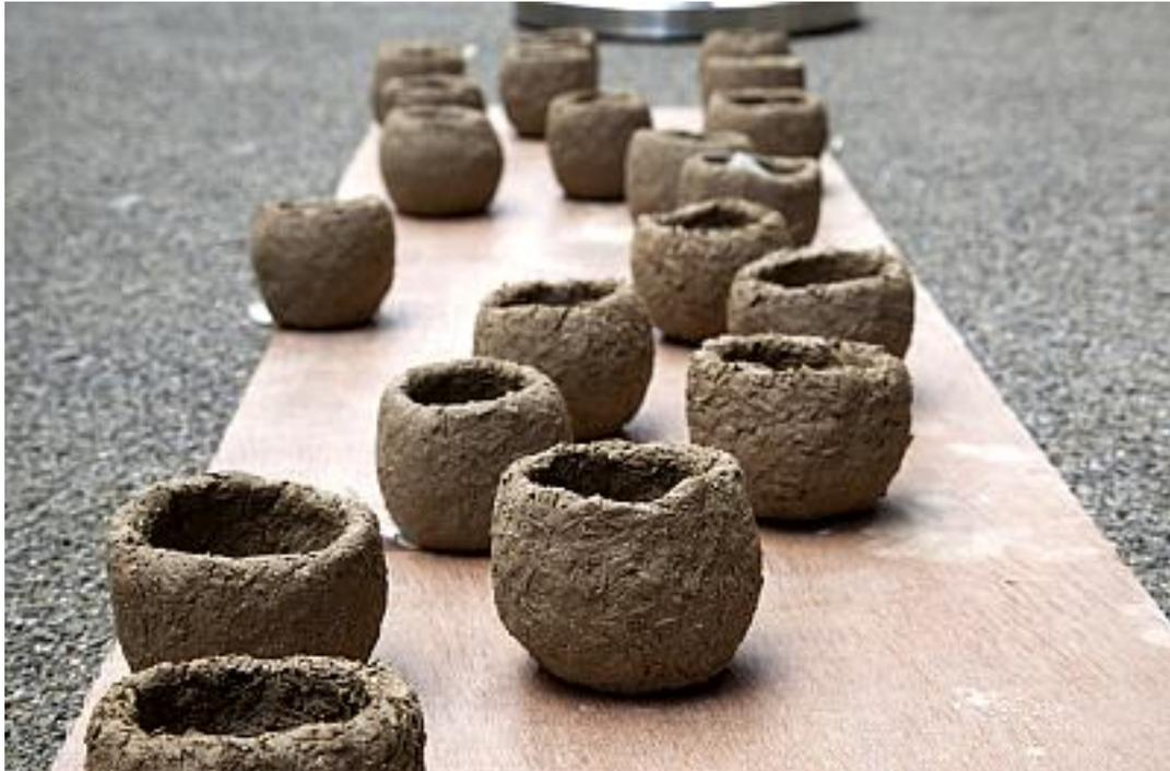
Day 3: To make bronze you can use a few different 'recipes', some include arsenic or lead to modify the properties. For obvious safety reasons, we used plain copper and tin. We used 10 times the weight of the wax in copper, and we could choose to either use 10% or 20% of tin (20% would give make your object harder). Once measured and weighed with great accuracy, we joined the crucibles to the objects using another layer of the clay and rice husk mix. These were then left to dry overnight.
