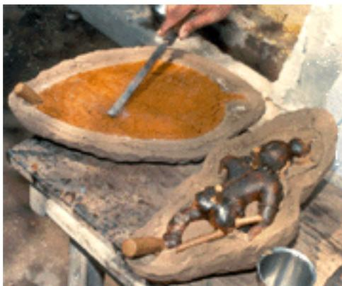
Figure 2. Completed mold halves with patterns after sun drying readied them for mold halves.
